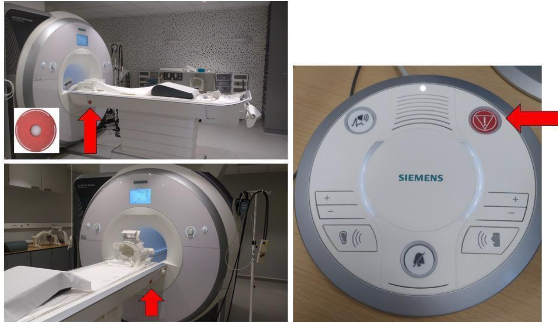
Figure 8: At top and bottom left, the Scanner Room Table Stop buttons. At right, the Control Room/Zone 3 Table Stop button. Note: to reset, press button at the back of the intercom console.
