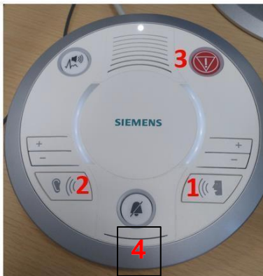
Figure 7: Siemens Prisma Fit intercom: 1) The Zone 3 speak mode button (must be held in continuously to speak to the participant and released to hear the participant). 2) The listen button (will pick up both the participant’s voice and the scanner noise). Press once to hear continuously and press again to end. 3) The Table Stop button. 4) The squeeze bulb alarm button (push once to end the alarm).
